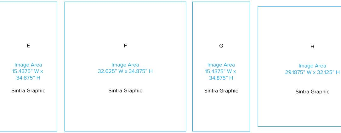
Sintra Infill Note:1/4" of graphic perimeter is hidden by extrusion
